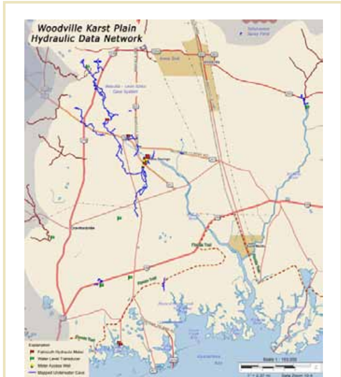
Map showing the location of hydraulic meters and water level transducers in the WKP.
