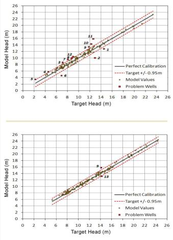
Calibration plots showing a match to within 1 m of target heads at 176 of 188 wells in region for the low water scenario (top) and 186 of 188 wells in the region for the high water scenario (bottom).
