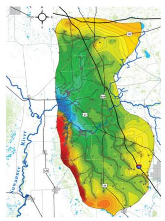
Model simulated low-water groundwater levels and location and pattern of simulated karst conduits (gray lines) relative to the river and wells used for calibration.
