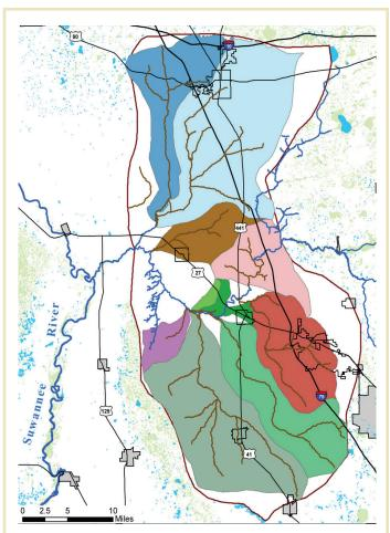
Model domain showing the delineation of individual springsheds from particle tracks exported from the low water scenario model run. This is the first numerical model to effectively delineate individual springsheds.
