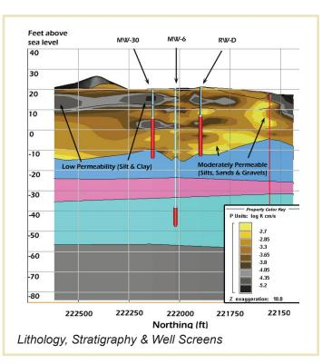
formed to determine how dissolved-phase VOCs will migrate through the surficial aquifer away from the LNAPL and the extent to which contamination may travel vertically into a lower potable aquifer.
