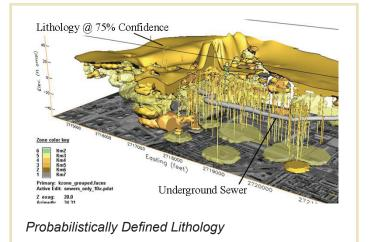
was then used to map hydraulic conductivity heterogeneity relative to underground structures and synoptic models of LNAPL morphology.
