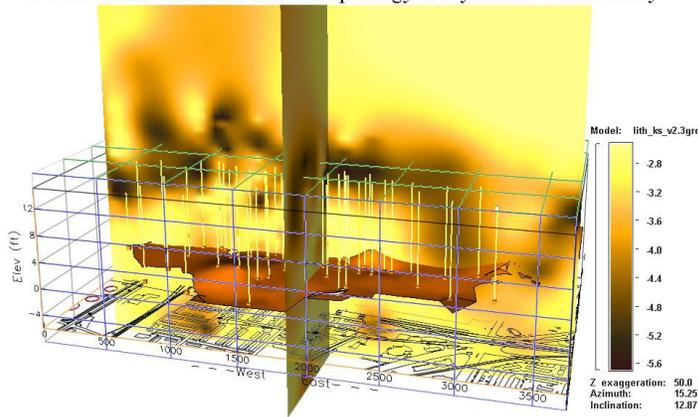
*Figure 3. Visualization of a 3-D LNAPL morphology model relative to the hydraulic conductivity, Defense Support Center Philadelphia, Philadelphia, Pennsylvania. The LNAPL plume is depicted as the rust-colored shape along the x-axis. The position of the silt layer is marked by the dark band above the LNAPL plume. Plume thickness is modeled to less than 0.01 feet. Vertical exaggeration is 50 times.*
