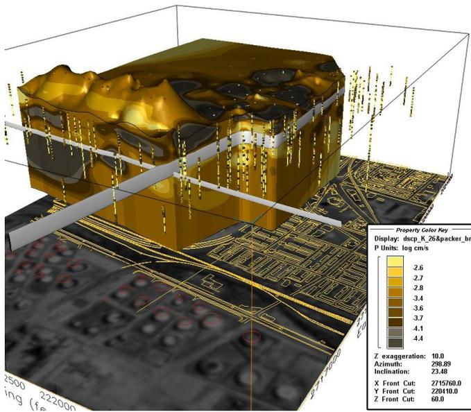
Figure 2. Visualization of 3-D hydraulic conductivity sliced along the Packer Avenue and 26<sup>th</sup> Street Sewers, Defense Support Center Philadelphia (DSCP), Philadelphia, Pennsylvania. View is from southeast to northwest across the 26<sup>th</sup> Street sewer. Vertical exaggeration is 10 times.
