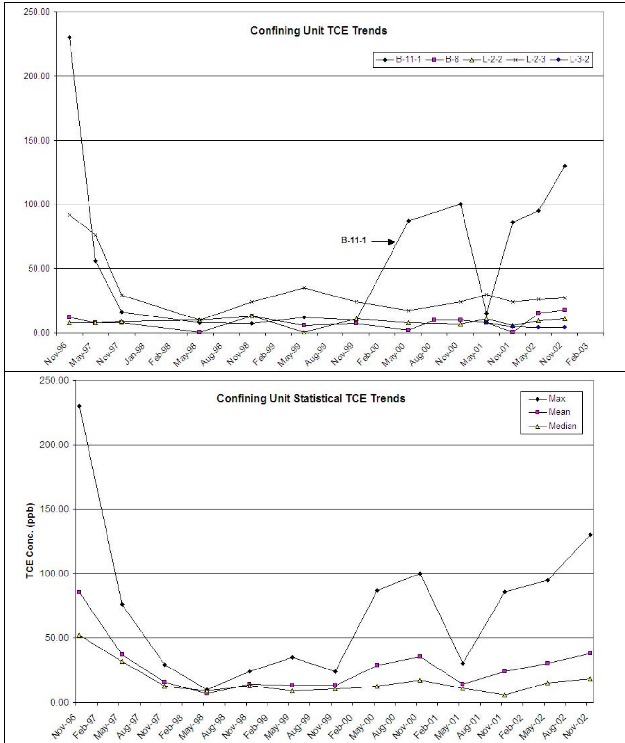
Figure 4. TCE concentration trends in confining unit monitoring wells at the Moltech facility, Alachua Florida between Nov. 1996 and Nov. 2002. (A) Trends in measured concentrations at all confining unit monitoring wells. (B) Trends max, mean and median values for all measurements on each synoptic period. Concentration trends in all but well L-2-3 and the max, median, and mean values indicate that the plume in the confining unit has been persisting and growing during the period of record, particularly in the vicinity of well B-11-1.
