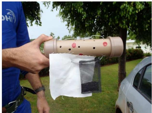
Figure 4. Aggregate charcoal and cotton samplers deployed at 12 of the 17 mine sampling stations.
