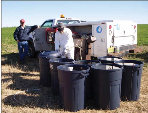
Filling chaser water into containers prior to injection.
