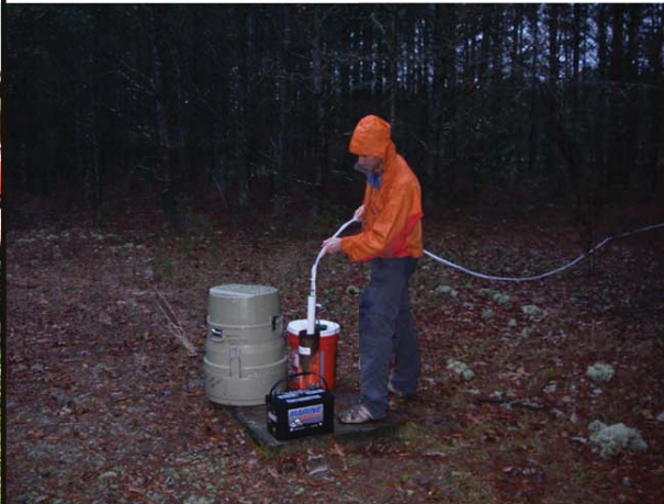
Installing pump and tube into monitoring well for sampling.
